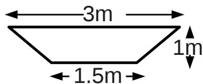
The diagram above shows the cross-section of a flood drainage trench.
